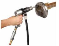
Remove all rust, mill scale and other foreign matter from the inside and outside of the tubes.
