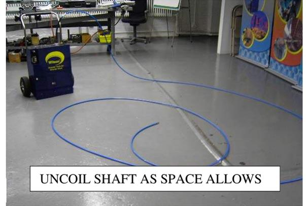
UNCOIL SHAFT AS SPACE ALLOWS
