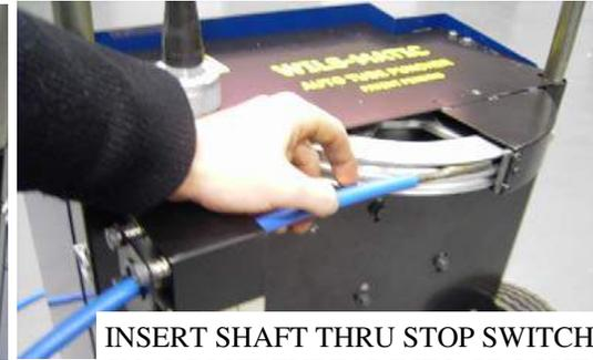
INSERT SHAFT THRU STOP SWITCH & SNAP BLUE TUBING INTO GROOVE
