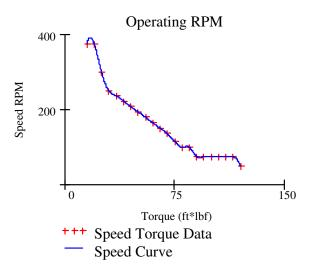
Table 4: Torque vs RPM chart (with POT reference marks)
