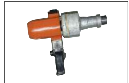
The 22488 Electric Rolling Motor rolls tubes up to 3-inch Outer Diameter.
