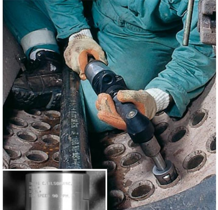
*The 909 Torque-Controlled Rolling Motor has the ability to control the torque, simply by adjusting this dial ranging from 150 to 305 ft.-lb.*
