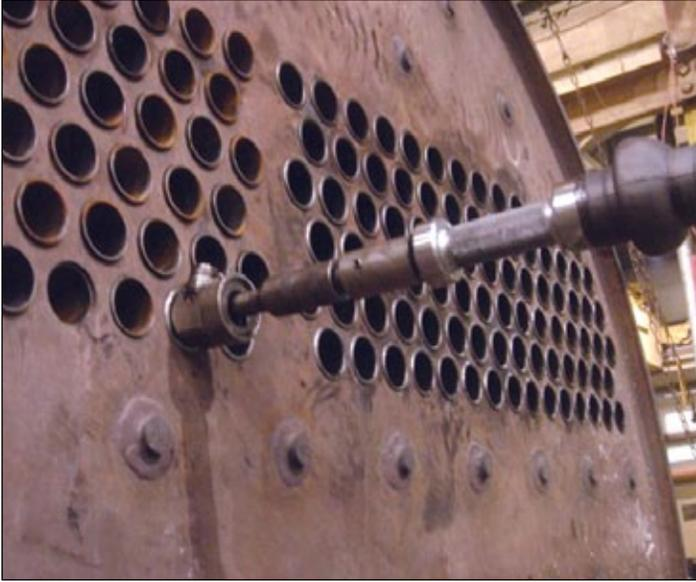
The Wilson Combination Beading Expander is one of our smartest tools! Rather than expand a tube, then manually bead it and then re-roll it with a straight roll expander, the patented Combination Beading Expander (CBE) from Thomas C. Wilson does all three jobs in one seamless process.
