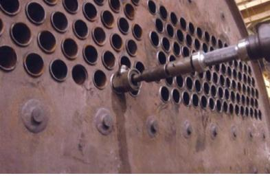
The Wils-Away<sup>™</sup> 1000 Cleaning a Fire Tube Boiler
